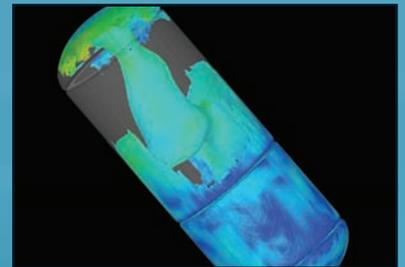
*Liquid fluorine tank under low gravity coast during launch.*
