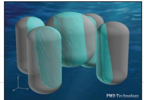
Simulation of fuel sloshing in a nutation 5-tank configuration at mid-range spin rate.
