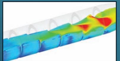
*Transient velocity magnitude contours of sloshing in aircraft fuel tank through a turn under acceleration.*
