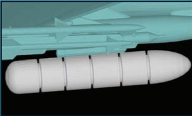
*FLOW-3D's* FAVOR™ method makes accurate representation of complex geometries simple.
