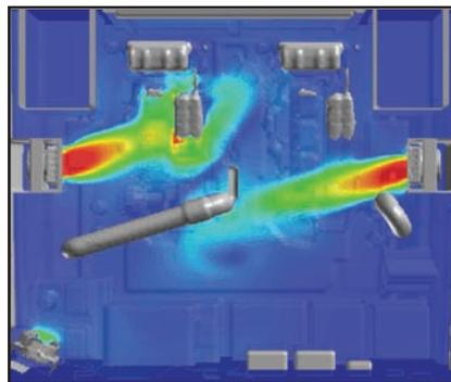
Ventilation of engine compartments, especially where heat generation can affect both performance and comfort, can be crucial in aerospace designs. **FLOW-3D** has been used to improve the efficiency of cooling systems and maintain a specified temperature in the interior compartments and a maximum internal average temperature.
