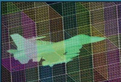
ADT decomposes the domain for balanced processor loads.
