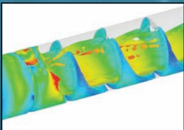
*FLOW-3D's* TruVOF technique provides accurate representation of fuel sloshing and fluid breakup.
