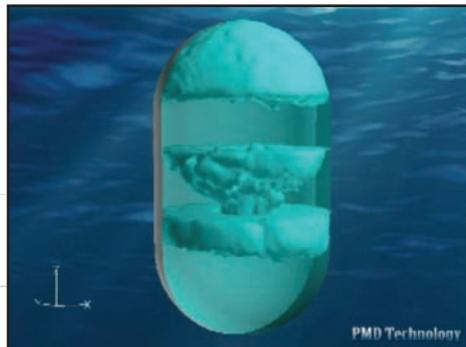
Vapor bubble migration in a baffled tank subject to a short engine firing.
